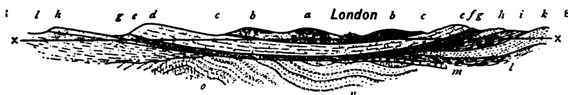
Fig. 21.—Generalised section across the London Basin, from north to south, showing the underground range of older rocks. a , Bagshot Sand (of Hampstead); b , London Clay; c , Lower London Tertiaries, Oldhaven and Blackheath Beds (on the south only), Woolwich and Reading Beds, Thanet Sand (on the south only); d , Upper Chalk; e , Middle and Lower Chalk; f , Upper Greensand; g , Gault; h , Lower Greensand; i , Weald Clay; l , Hastings Beds; l , Middle and Upper Jurassic Beds; m , Lower Jurassic Limestone with clay in the centre; n , Red Rocks and Devonian (possibly with Carboniferous in places); o , Silurian; xx , Sea-level. Vertical scale exaggerated.
